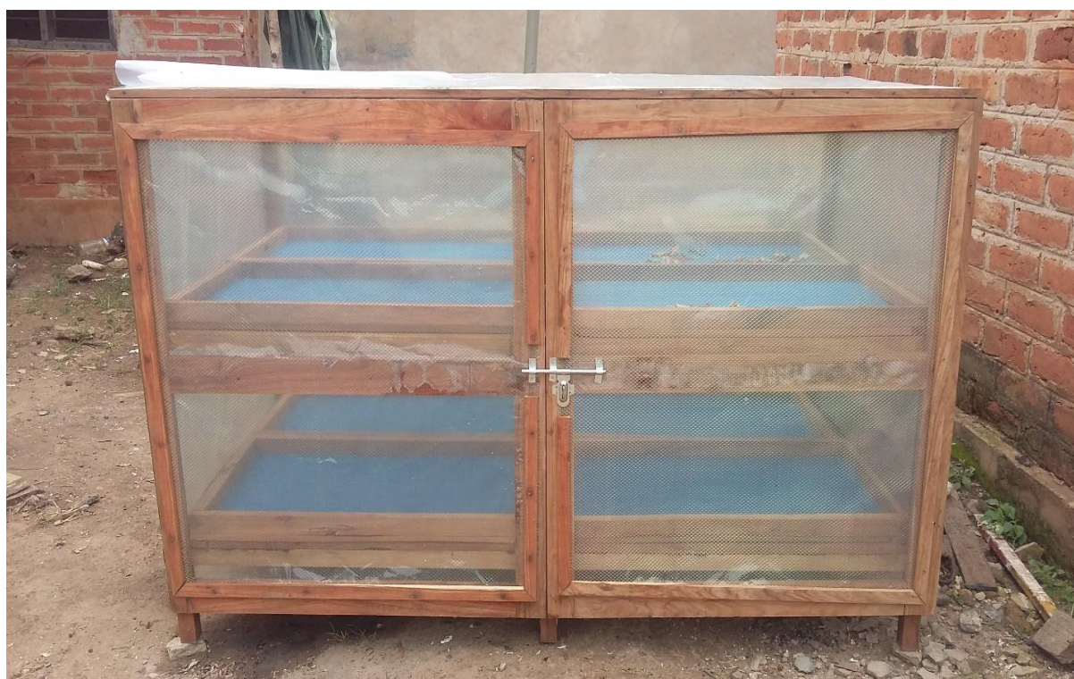
Fig.4. Locally made movable and simple solar dryer from Inyonga.
