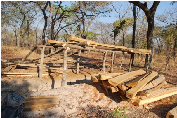
Pit-sawing for timber logging (Stampfli, 2016)
