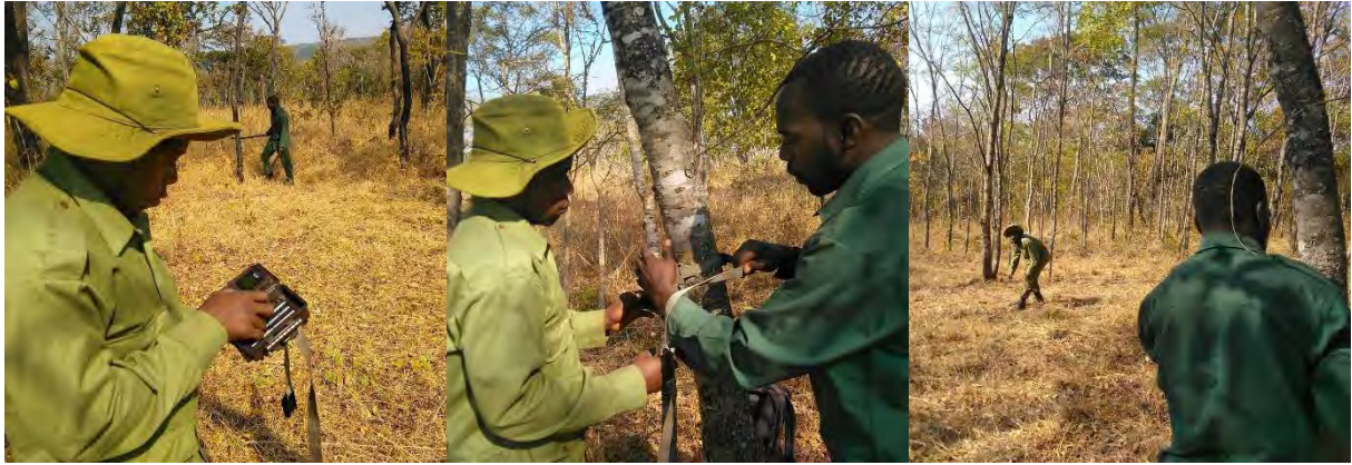
Figure 16: Installation of a CT in the field. First, configure the CT. Second, set-up the CT on the chosen tree. Third, trigger the CT ("test mode) to verify CT functioning properly
